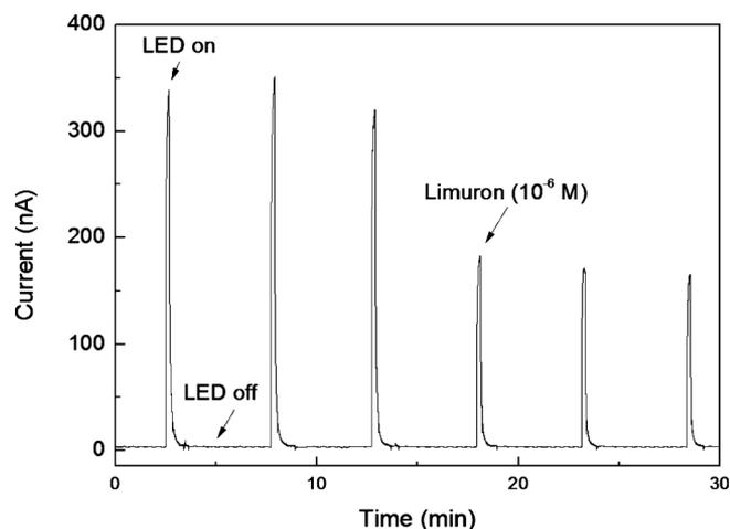
FIG. 3. Herbicide inhibition, as chronoamperometric measurements, of the spinach thylakoids immobilized onto gold SPE. The herbicide (Linuron  $10^{-6}$  M) has been added after three light pulses. The duration of light pulses was set to be 5 s with a frequency of 5 min.
