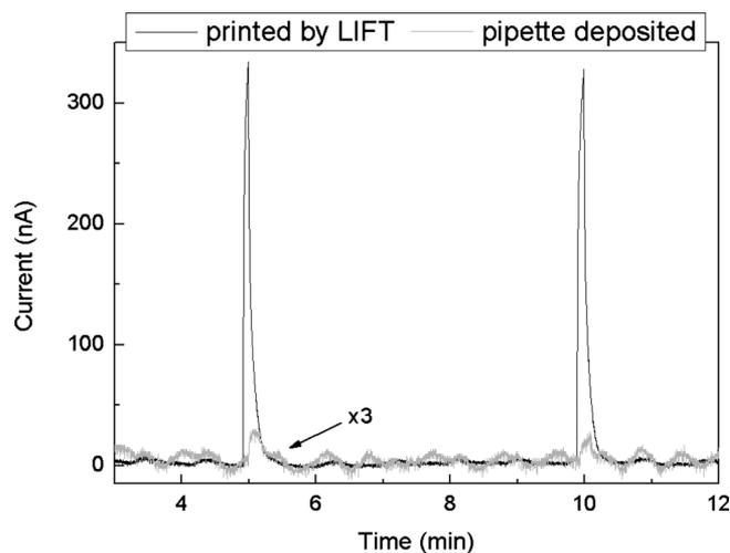
FIG. 2. For comparison, typical electrical signals for printed by LIFT (black line) and pipette deposited (gray line) sensors.
