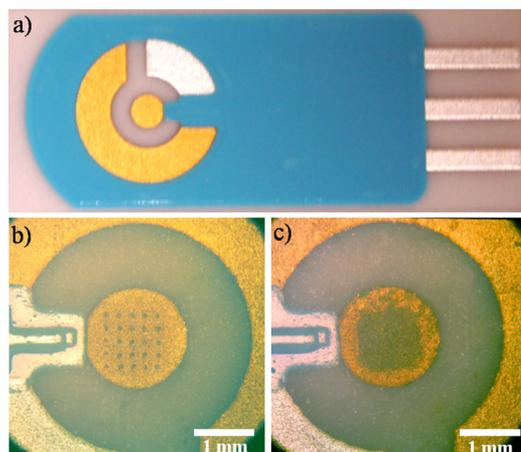
FIG. 1. (Color online) (a) A picture of a gold SPE (Dropsens C223AT) sensor. (b) Discrete thylakoid pixels printed by LIFT on the working electrode of the SPE sensor. (c) A continuous thylakoid layer printed by LIFT on the working electrode of the SPE sensor.
