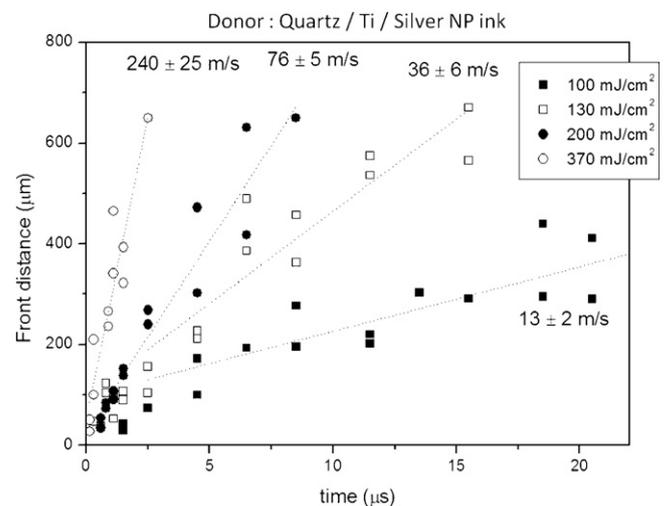
**Fig. 3.** Titanium layer assisted LIFT of silver NP ink. Plot of the front material position as a function of the time delay with respect to the pump laser pulse. The standard error of the slope was used to determine the corresponding standard error for the velocity.
