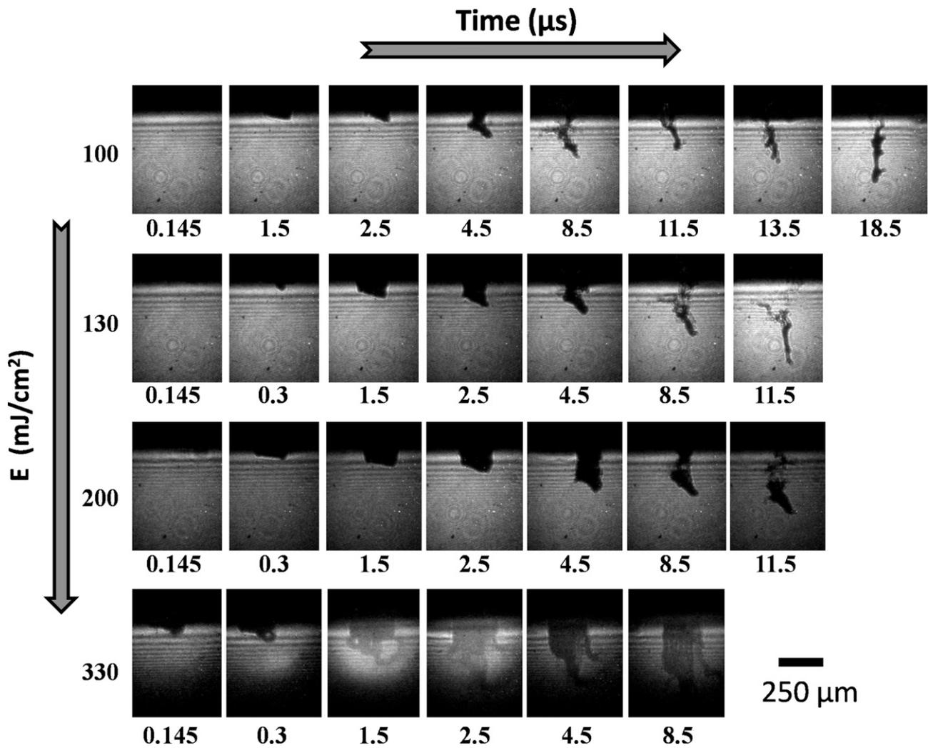
**Fig. 2.** Shadowgraphic time-resolved images of the silver NP ejection using titanium DRL assisted LIFT for various laser fluences. Pictures were taken at different time delays with respect to the pump laser pulse.
