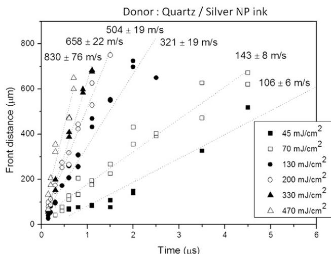
**Fig. 5.** LIFT of silver NP ink without using DRL. Plot of the front material position as a function of the time delay with respect to the pump laser pulse. The standard error of the slope was used to determine the corresponding standard error for the velocity.
