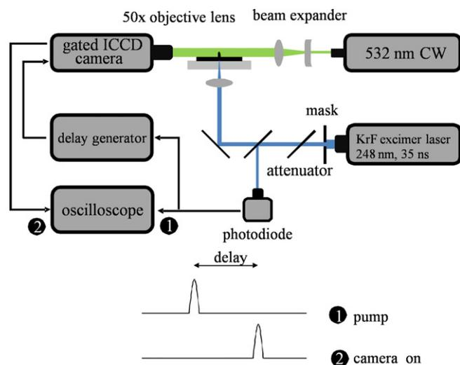
**Fig. 1.** A sketch of the shadowgraphic time-resolved imaging setup. A pump KrF excimer laser (248 nm, 35 ns) initiates the ejection of silver NP ink. The images are captured with a gated ICCD camera, which is synchronized to the pump laser through a photodiode and a pulse delay generator. Both photodiode and ICCD signals were sent to an oscilloscope for accurate measuring of the delay time.
