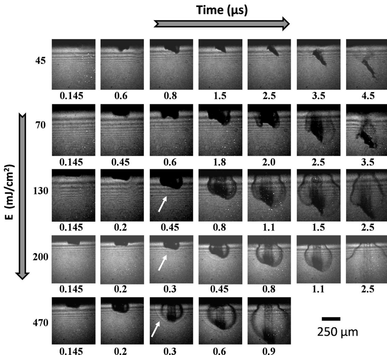
**Fig. 4.** Shadowgraphic time-resolved images of laser transfer (without titanium DRL) of silver NP ink for various laser fluences. Pictures were taken at different time delays with respect to the pump laser pulse. The laser fluence of 130 mJ/cm<sup>2</sup> is the threshold for a shock wave propagation, which is indicated by white arrows.
